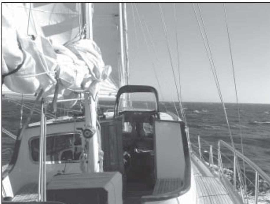
The mizzen aboard this 82-foot ketch, under delivery by Adam Smith of Echo Yacht Deliveries, has been reefed to balance out the sail plan as the crew makes its way south to Mexico. Smith told us that 'keeping friction and chafe to a minimum' are the most important factors in making a reefing system perform. For that, he prefers roller-bearing blocks, which are hidden in this photo by the reefed portion of the sail
